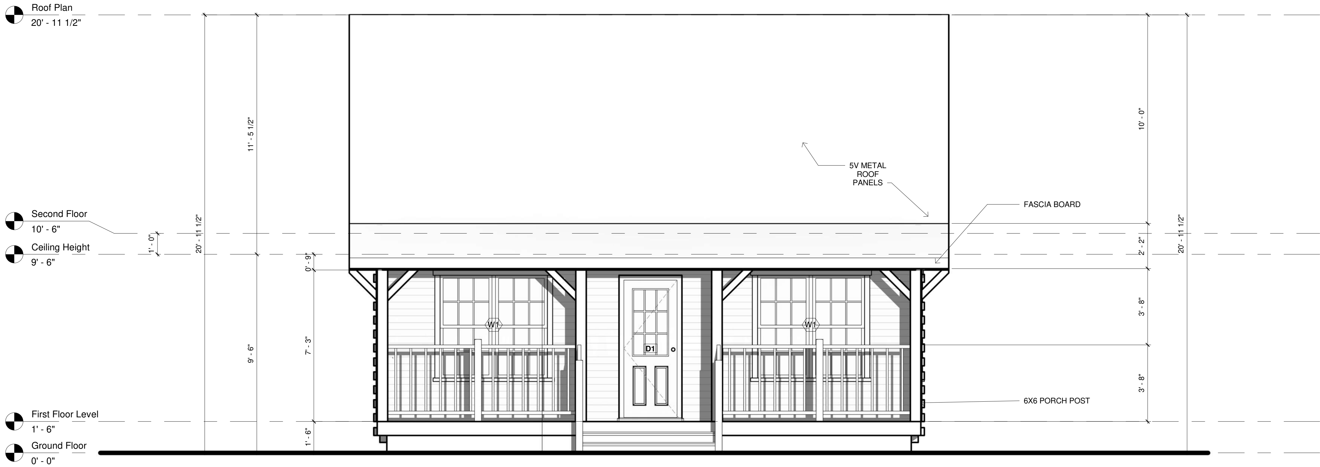
SOUTH EXTERIOR ELEVATION
